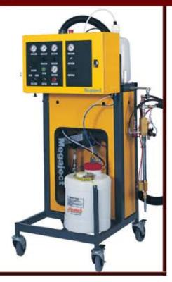
Designed for injecting Polyester resins and catalyst at controlled pressures, this machine mixes on demand at the injection head.
