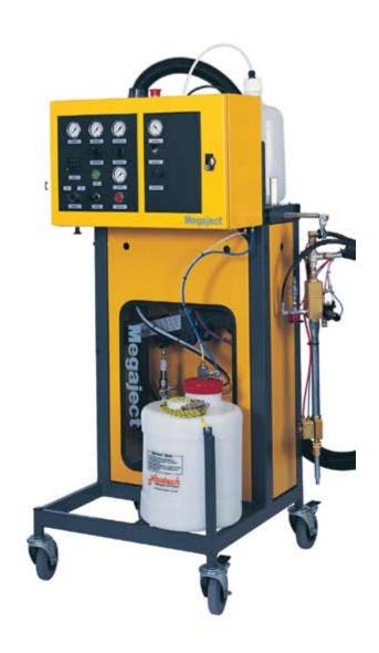
Suitable for Injection of Polyester, Vinylester and Methacrylates **Built-In Pneumatic Interlocks** Resin Gel Alarm (RGA)
