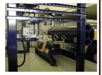
Versatility to meet your future demands: The Magnum Venus Plastech Programmable **Ultra-Winder** is the most versatile filament winder on the market today. Modularly constructed to grow with your changing production needs, both chop-hoop and helical winding of various pipes and tanks can be performed by this computer-controlled machine.
